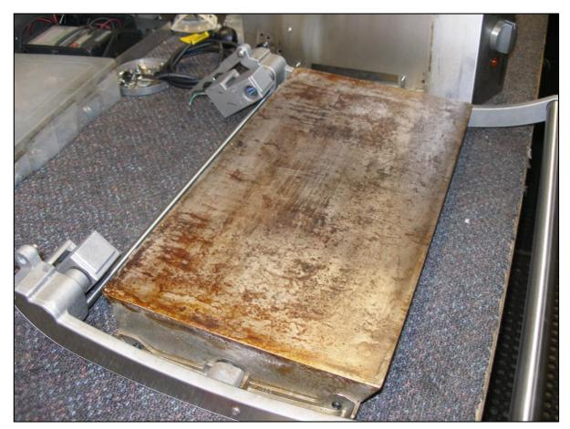
After removing the bottom plate you will be left with the top plate connected to the side handles and the bush mounting blocks on the bench.
