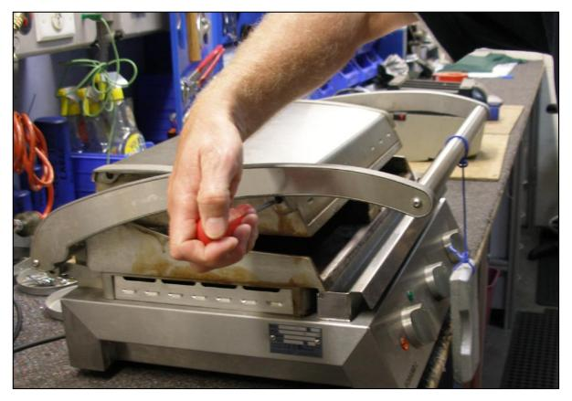
Having the spacer between the plates allows access to the screws holding the aluminium cover pieces for the stainless steel top. Remove the two screws from each side.
