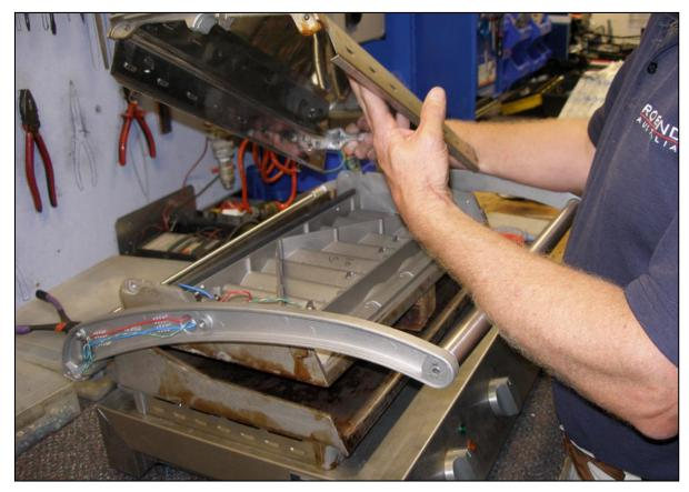
Remove the top stainless steel cover; you may need to use a flat blade screwdriver to lightly tap the top cover retainers outwards which will allow separation to occur.
