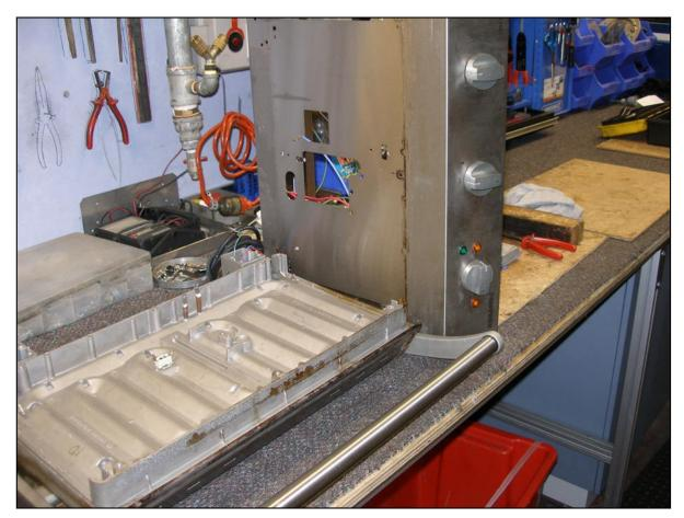
Place the stainless steel body to the right of the plate on its end.
