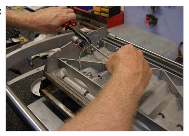
Unscrew the wires connected to the terminals of the element in the plate but ensure you hold the terminal with pliers to prevent it from twisting when doing so. Once this is completed the top plate can be removed by lifting the handle with the counter weight up approximately 50mm and sliding the plate forwards and off the spacer.
