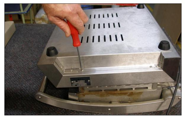
The machine should be placed in the upside down position allowing access to the bottom cover. Remove the six base screws; it is not necessary to remove any of the other screws on the underside.
