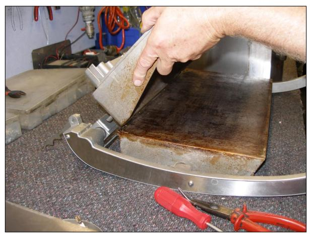
Grasp the bottom plate with both hands and manoeuvre it off past the two rear aluminium posts and the top plate.
