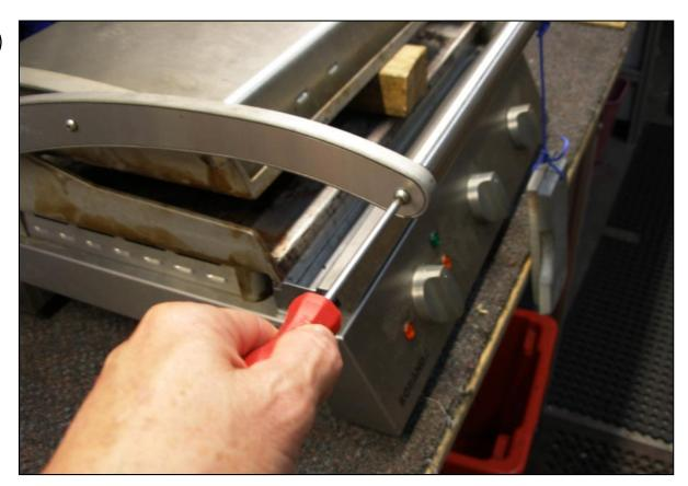
Loosen the screw in the front handle approximately 3 turns to reduce the tension on the top stainless steel cover.
