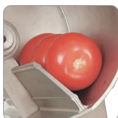
Stacking of Tomatoes on Cylinder Wall
