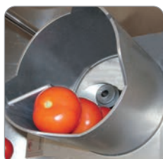
Stacking of tomatoes on cylinder wall
